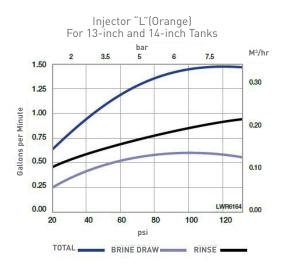
\*New injectors for high-efficiency regeneration sequence are standard with Logix Controllers. NOTE: Actual injector performance is dependent on the resin used, tank geometry, elevated drain, etc. This injector data was taken using an empty tank (no resin).
